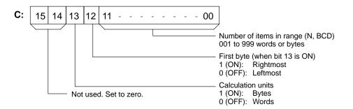
Number of Items in RangeThe number of items within the range (N) is contained in the 3 rightmost digits of<br/>C, which must be BCD between 001 and 999.
